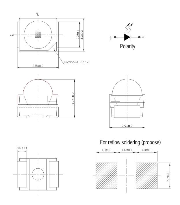
**Notes:** The tolerances unless mentioned is  $\pm 0.1$ mm ,all dimensions are in millimeters.
